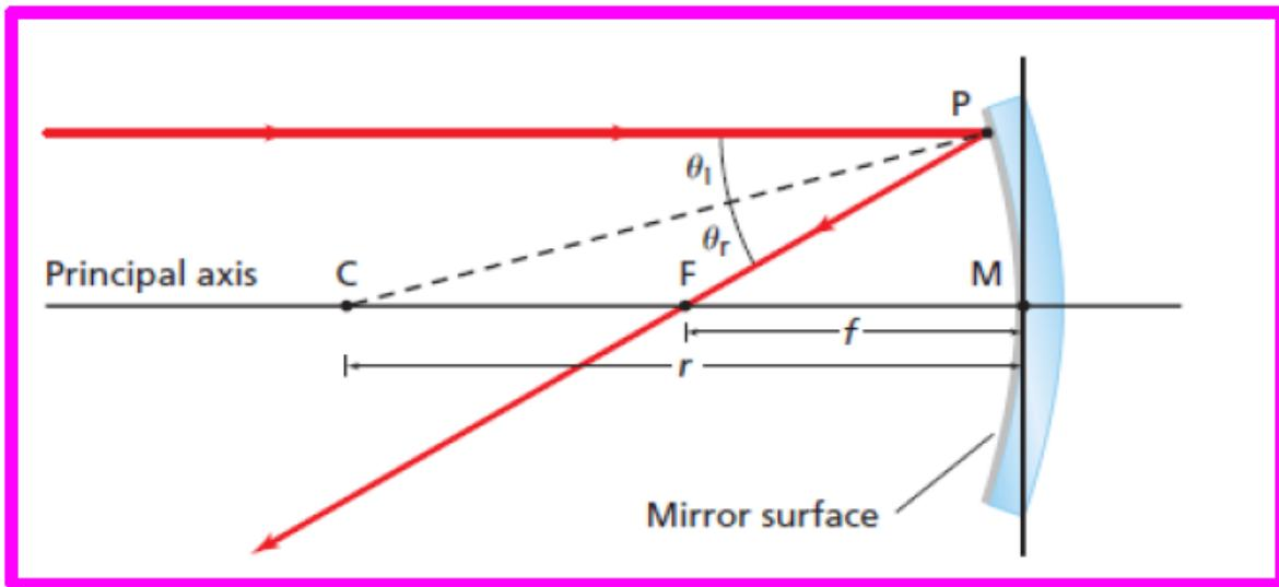
The relationship between the focal length and the radius of the curve
