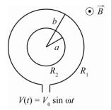
**RESEARCH:** The current through the large loop is  $I = \frac{V_0 \sin \omega t}{R_1}$ . This creates a magnetic field at the center of the loop of:
