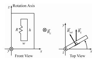
**RESEARCH:** The induced current, *i*, is found from  $i = V_{ind} / R$ , where  $V_{ind}$  is given by  $V_{ind} = -d\Phi_B / dt$ , and  $\Phi_B = BA \cos\theta$ . As the door opens, the B field through the loop decreases; by Lenz's law the induced B field points into the page, at an angle of  $\theta(t)$  from the plane of the page. The induced current flows clockwise.
