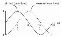
**29.34. THINK:** The varying current,  $i_1$ , through the outer solenoid creates a varying magnetic field,  $B_1$ , within the coil. This varying *B* field creates a flux in the inner solenoid, which in turn creates an induced *emf*. **SKETCH:**
