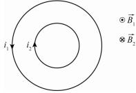
**RESEARCH:** The magnetic field generated by the outer solenoid is given by  $B_1 = \mu_0 n i_1 = \mu_0 n i_0 \cos \omega t$ . The flux generated in the inner solenoid is given by  $\Phi = A_2 B_1$ . The induced emf in the inner solenoid is given
