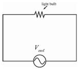
**RESEARCH:** The average power of the bulb is  $\langle P \rangle = I_{\rm rms}^2 R$ . The rms voltage is  $V_{\rm rms} = I_{\rm rms} Z$ , where  $Z = \sqrt{R^2 + X_L^2}$  and  $X_L = \omega L$ .
