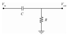
**RESEARCH:** The signal ratio is  $V_{\text{out}} / V_{\text{in}} = 1 / \sqrt{1 + 1 / (\omega^2 R^2 C^2)}$ , where the angular frequency is  $\omega = 2\pi f$ . SIMPLIFY:  $\sqrt{$
