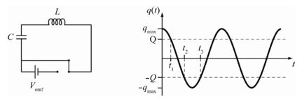
**RESEARCH:** The initial (and maximum) charge on the capacitor is  $q_{\text{max}} = CV$ . The charge will oscillate as  $q = q_{\text{max}} \cos(\omega_0 t)$ , where  $\omega_0 = 1/\sqrt{LC}$ .
