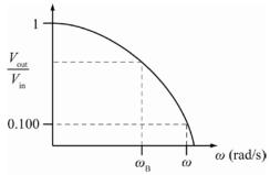
**RESEARCH:** For a RC low-pass filter, the breakpoint frequency is:  $\omega_{\rm B} = 1/(RC)$ , where  $\omega_{\rm B} = 2\pi f_{\rm B}$ . The ratio of the input voltage to output voltage is
