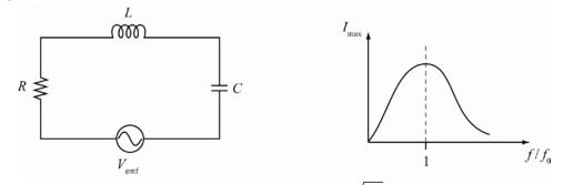
**RESEARCH:** At resonance, the angular frequency is  $\omega_0 = 1/\sqrt{LC}$ , where  $\omega_0 = 2\pi f_0$ . At resonance,  $V_R = V_{emf}$  and  $V_L = -V_C$ , where  $V_L = IX_L$ . Recall V = IR and  $X_L = \omega_0 L$ .
